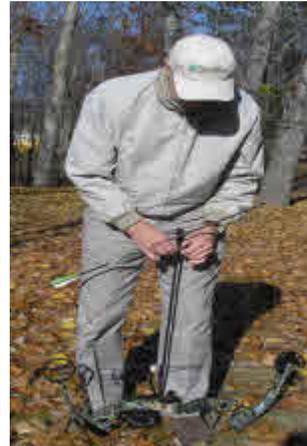
Draw the bow with both hands from a sitting position or standing with a foot stirrup. Drawing the bow in this manner allows a person to draw a bow of much greater draw weight than they could in a traditional manner. I always draw the bow with an arrow in my hand so I will not forget to nock one before firing. The Lock-a-Draw looks like an arrow when sighting.
