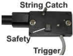
The Lock-a-Draw string catch is now cocked by a spring, and the safety is always on. To pull the trigger you have to depress the safety button and actuate the trigger. This is a great safety feature.
